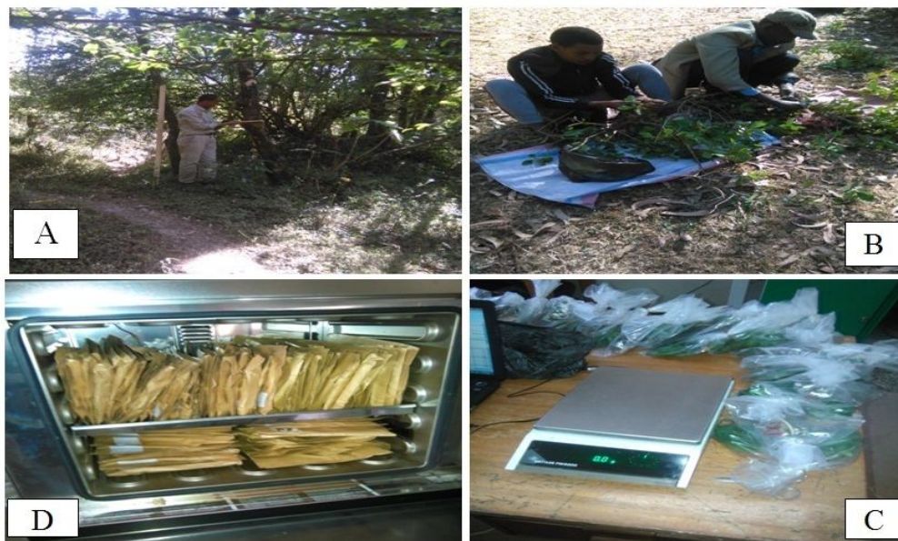
Figure 4: Tree DBH measurement (A), separation of sample leaves and branches (B), sample weight measurement (C) and oven drying subsamples (D)
