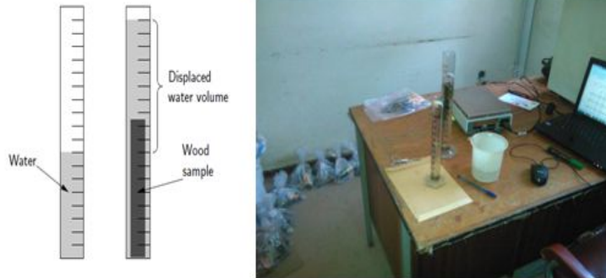
Figure 5: Measurement of sample fresh branch wood volume by water displacement.
