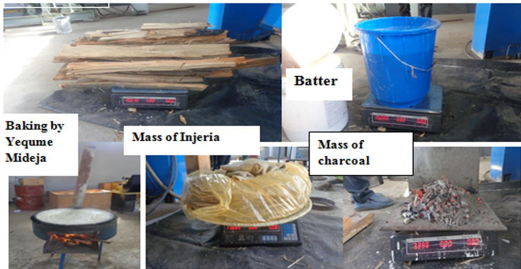
Figure 3-3:- Measurement technique during baking using digital balance
