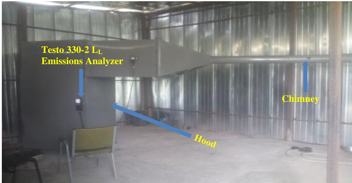
Figure 3.10: Total emission test on produced Khat residue briquettes
