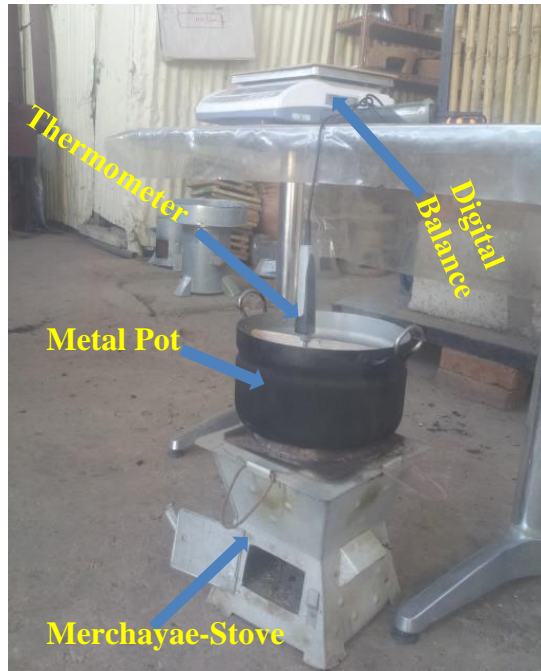
Figure 3:9: Combustion and Water boiling capacity test on produced briquettes
